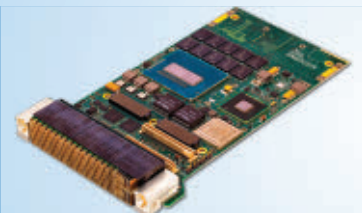
XPedite7570 4th Gen Intel® Core™ i7-based 3U VPX SBC with XMC/PMC
