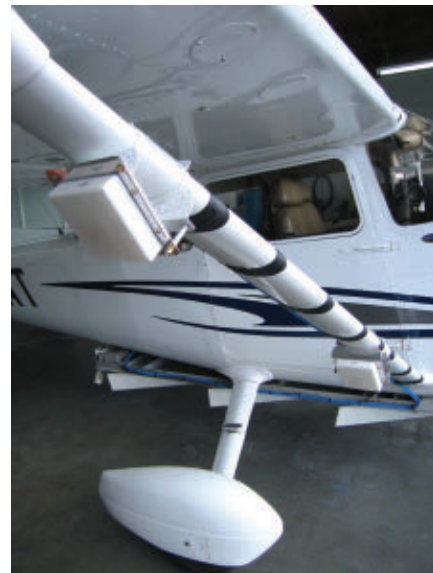
A national team of geotechnical engineers attached imaging equipment to the wing of a lightweight Cessna plane to collect data related to the recent Oso, Wa., mudslide.
