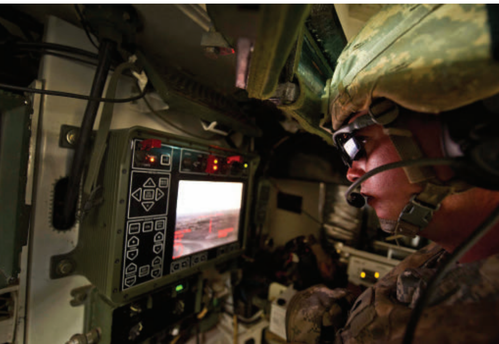
Vetronics displays enable combat vehicle crews to see outside the vehicle using signals from networked sensors.
